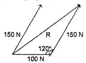
Placing the vectors head to tail combined with law of cosines produces R = 217.94.
